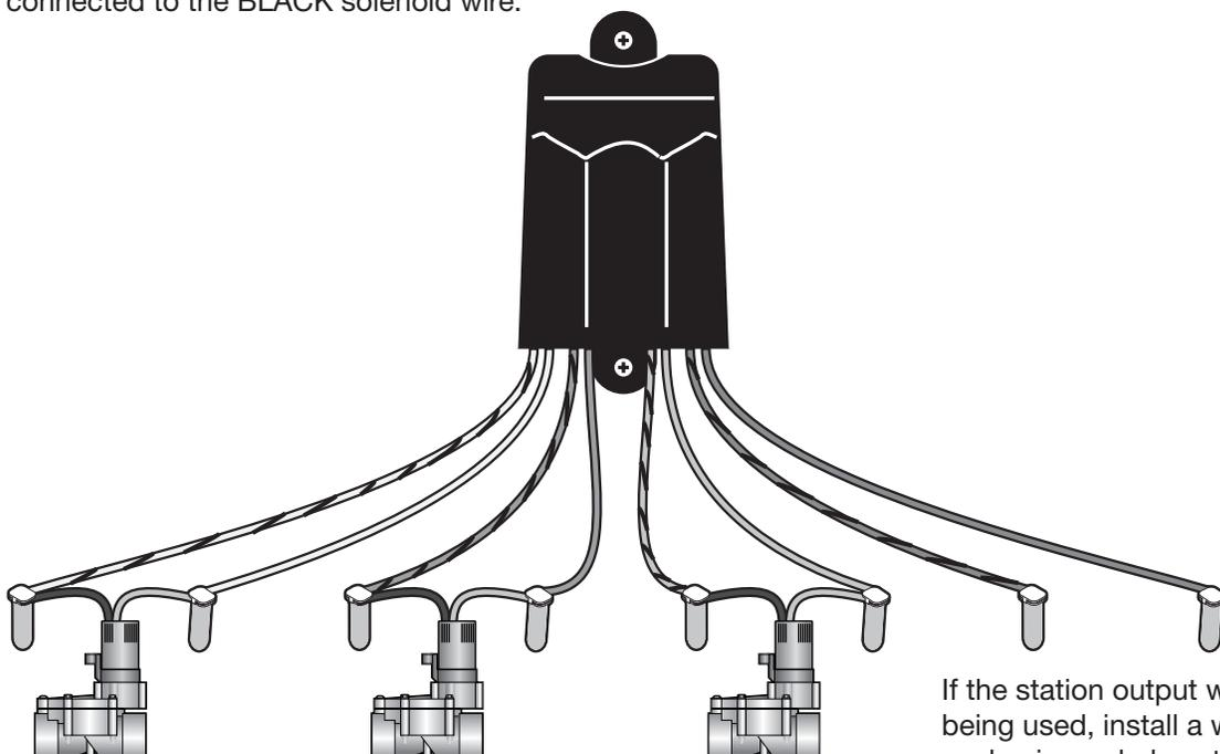
If the station output wires are not being used, install a wire nut on each wire and place them in a DBY.
