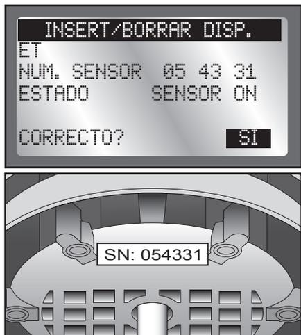
Si coincide, pulse
