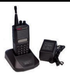
The Sentinel® remote allows users to conduct irrigation checks, and fully operate the system without opening a field satellite enclosure or needing a second person. This remote also serves as a two-way voice radio, allowing easy communication with other crew members.
