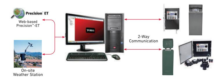
Maximize efficiency on your Sentinel system by using ET-Based watering. ET-Based watering automatically schedules irrigation based on individual landscape needs and local weather conditions. The result is higher property values, lower water bills and a healthier environment. Unlike competitive systems, Sentinel works in conjunction with multiple weather sources including on-site weather stations and Toro's wireless, web-based Precision $^{\mathsf{TM}}$  ET.
