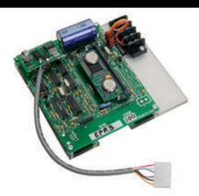
The Sentinel® Retro-Link assembly unit allows an existing Rain Bird® ESP-MC controller to be upgraded to a Sentinel field satellite. Retro-Link is 100% compatible with the Sentinel central control software.
